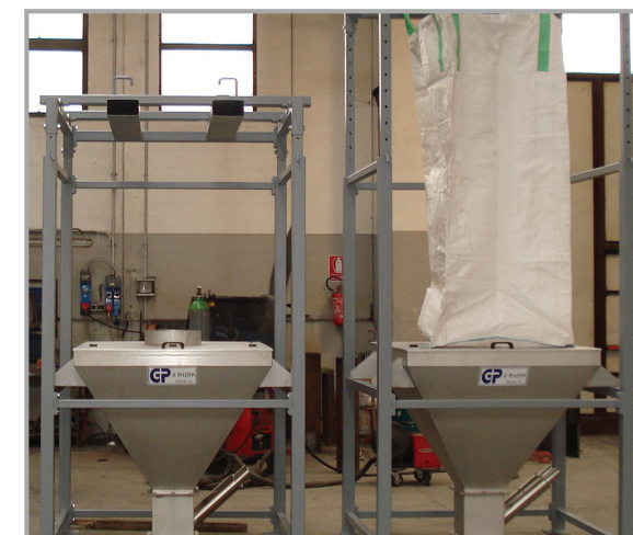
SVUOTA BIG-BAG CON CARICO TRAMITE CARRELLO ELEVATORE BIG-BAG EMPTYING WITH TRUCK LIFT LOADER
