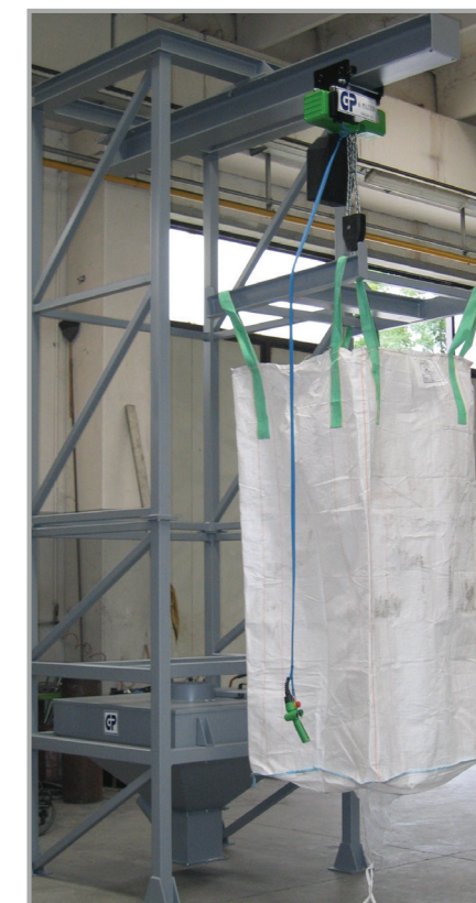
SVUOTA BIG-BAG TRAMITE PARANCO ELETTRICO BIG-BAG EMPTYING BY MEANS OF ELECTRIC HOIST
