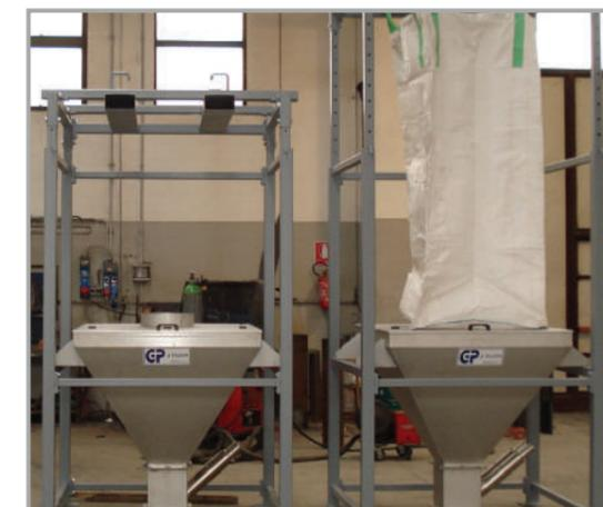
SVUOTA BIG-BAG CON CARICO TRAMITE CARRELLO ELEVATORE
