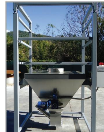
SVUOTA BIG-BAG CON CARICO TRAMITE CARRELLO ELEVATORE CON ROMPI PONTE
